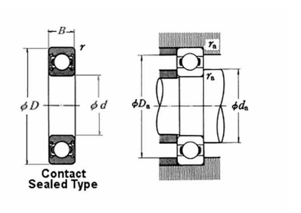
High quality Deep groove ball bearing with contact rubber seal on one side from the world leader NSK, the worlds largest ball bearing manufacturer offering unparalelled quality. The unique & patented NSK DDU rubber seal features market leading technology, keeping contaminants and moisture out of the bearing while retaining the high class lubricant inside
